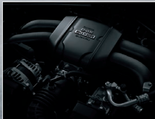
Horizontally-opposed Boxer engine
